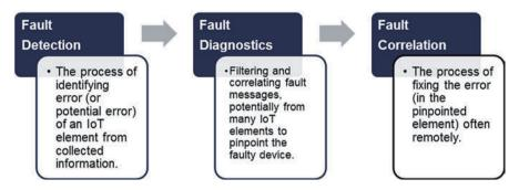
Fig. 7.7 Main stages of Fault Management function
