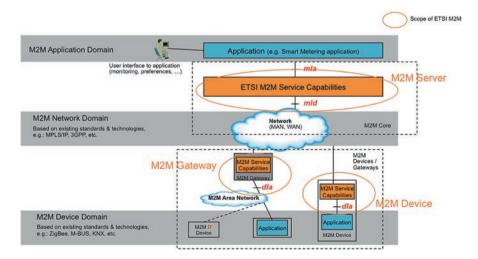
Fig. 5.20 ETSI M2M system architecture
