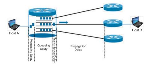
Fig. 2.7 End-to-end delay from host A to host B with illustration at router A
