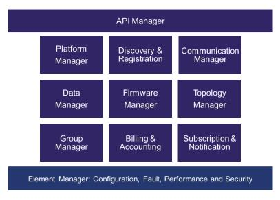
Fig. 7.4 Common IoT Services Platform Functions
