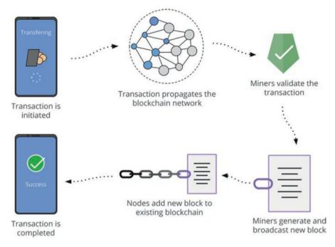
Fig. 10.4 How a Bitcoin transaction is executed
