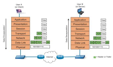
Fig. 2.2 Illustration of OSI model
