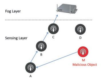
Fig. 8.9 Illustration of the stretch attack
