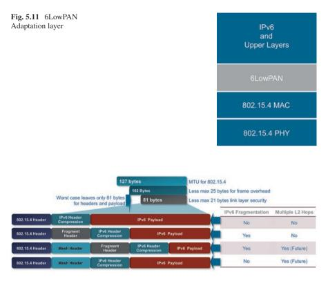
Fig. 5.12 6LowPAN header stack. (Source: Cisco BRKIOT-2020, 2015)
