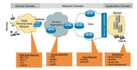
Fig. 5.18 ETSI M2M network architecture
