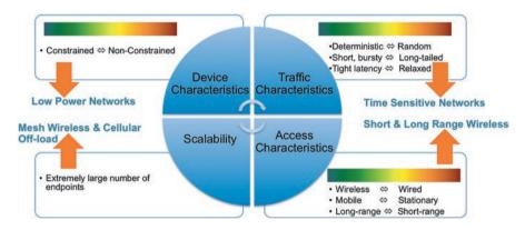
Fig. 5.2 Link layer challenges. (Source Cisco BRKIOT-2020, 2015)
