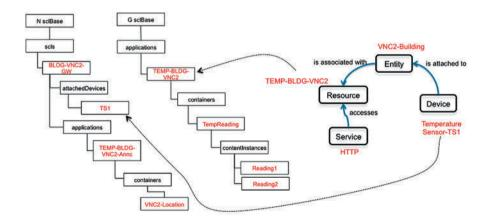
Fig. 5.19 Example ETSI M2M resource tree
