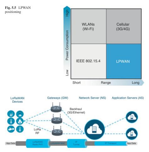
Fig. 5.6 LoRaWAN end-to-end network architecture
