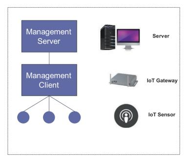
Fig. 7.5 Example of element management function
