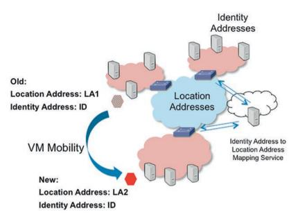
Fig. 6.3 Identity vs. location addresses with application mobility
