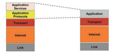
Fig. 5.1 IoT protocol stack
