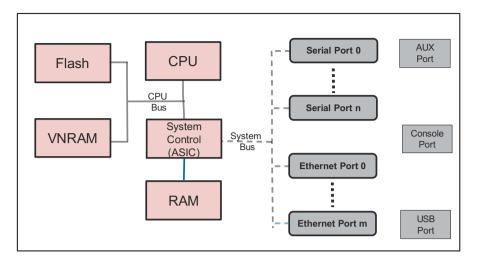
Fig. 2.4 Router main components
