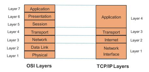
Fig. 2.3 Relationship between OSI reference model and TCP/IP
