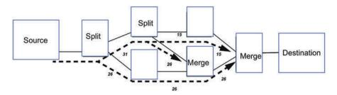
Fig. 5.9 IEEE 802.1CB seamless redundancy
